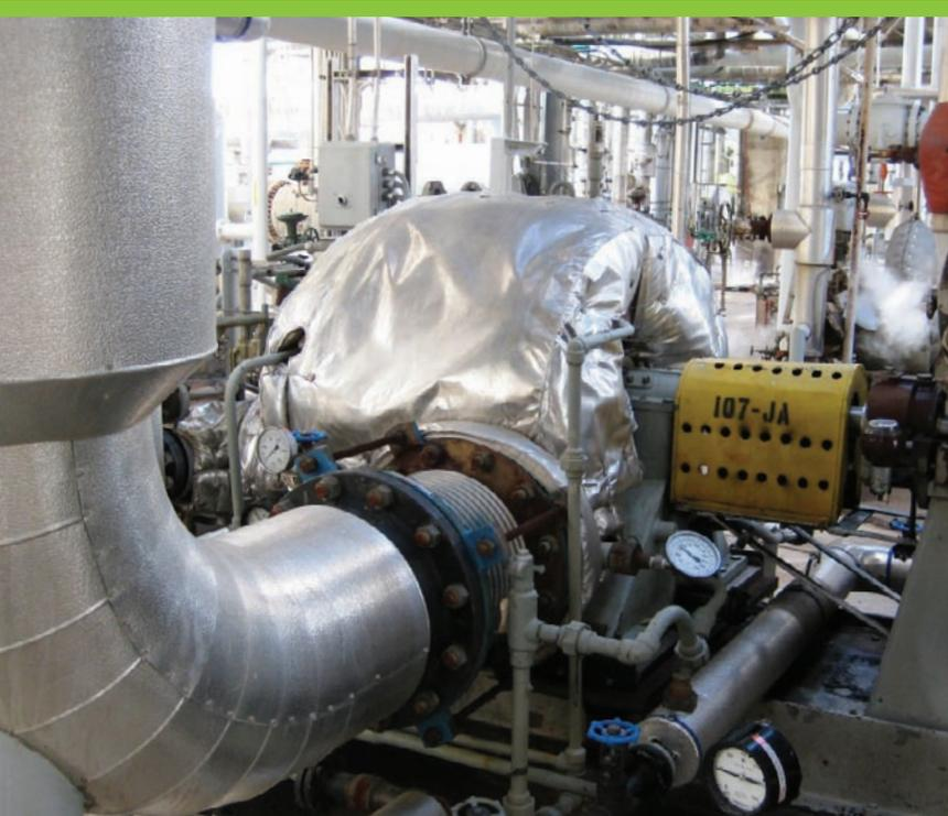
One of the new condensing turbines in ammonia plant #2; these new turbines are reducing energy use by 228,000 MMBtu annually.
