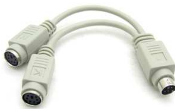
Figure 4-26 Y-Cable use for both Keyboard and Mouse
