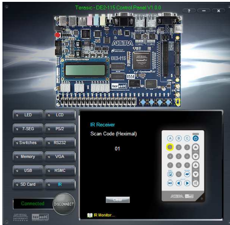
Figure 3-14 Testing the IR receiver using remote controller
