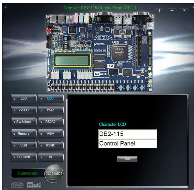
Figure 3-5 Controlling the LCD display
