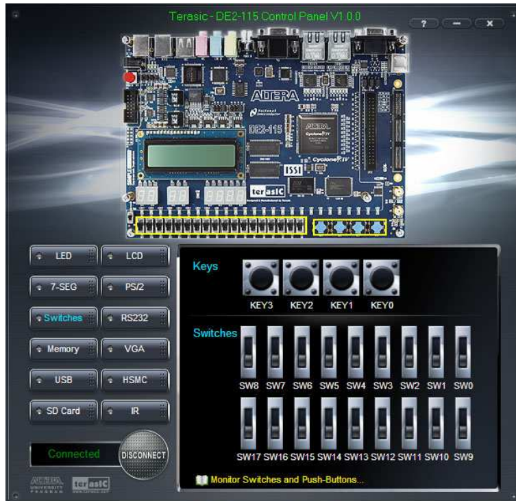
Figure 3-6 Monitoring switches and buttons
