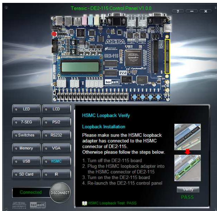
Figure 3-13 HSMC loopback verification test performed under Control Panel
