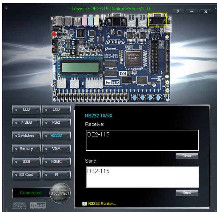
Figure 3-11 RS-232 Serial Communication
