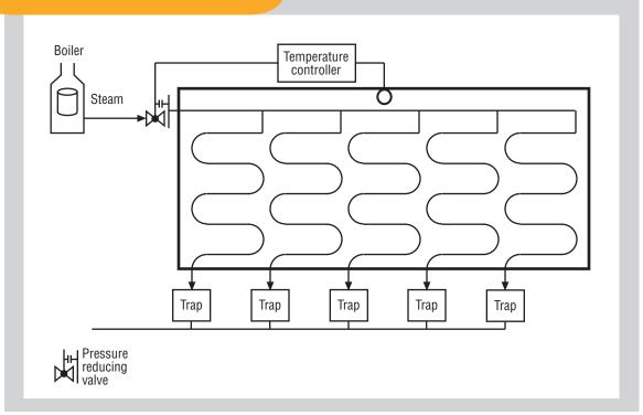
Sometimes an apparently minor piece of equipment in the overall system can actually be quite important. In this case, a poorly designed steam trap system led to a number of problems, resulting in inefficient operation of the entire process.
